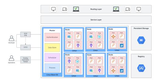
To ensure workloads (and the environment itself) are designed in a resilient and secure manner, it is important to understand the basic mechanics of how Kubernetes allocates & schedules deployments. This is particularly important because there are many configurable parameters that impact how and where workloads are scheduled and deployed.
